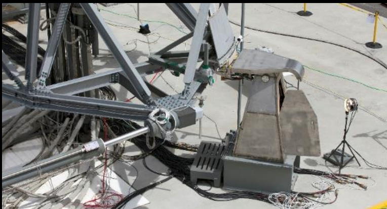
Aft Skirt Electrical Umbilical
